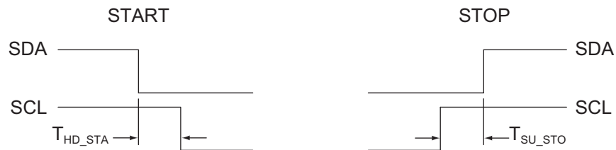
Figure 2: I²C Start and Stop Conditions; START: A High "1" to Low "0" Transition on the SDA Line While SCL is High "1" STOP: A Low "0" to High "1" Transition on the SDA Line While SCL is High "1."
